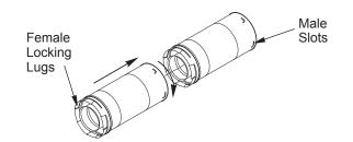
Figure 8 - Vent Pipe Connections
